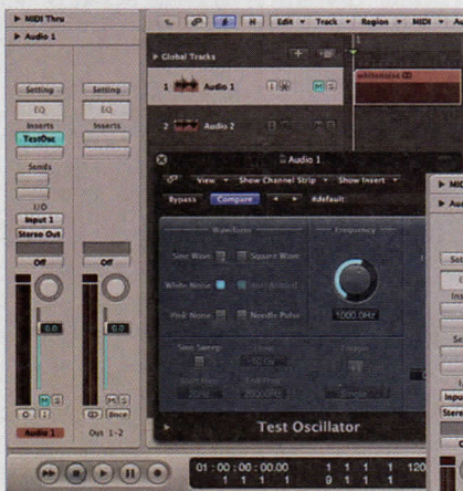
Step 1. Insert Logic's Test Oscillator plug-in on an audio track, and record some white noise directly into that track.
