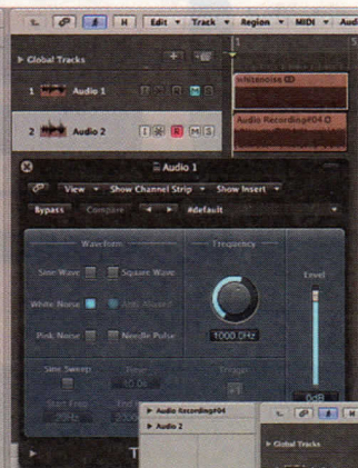
Step 2. Play back that track, and using a mic you know has a flat response, re-record this noise from your speakers onto a second audio track. Hold the mic where your head would be when mixing.
