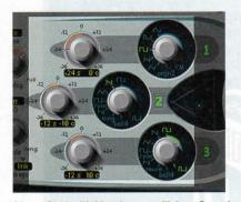
Step 1. Start with big, chewy oscillators. Osc 1 is set to a square wave, Osc 2 is a sawtooth, and Osc 3 is set up for pulse width modulation (see next step). Osc 1 is tuned -24 steps (two octaves down), and Osc 2 and 3 are tuned to -12, putting them an octave above Osc 1. Oscs 2 and 3 are also tuned up and down 10 cents, respectively, for some natural chorusing.
