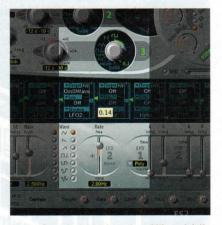
Step 2. Osc 3 is set up for pulse width modulation. PWM lets you affect the width of a pulse wave using a modulation source to add timbral and pitch animation. Here I've set LFO2 to a triangle wave at 2.0Hz, and have it modulating the pulse width of Osc 3's waveform.
