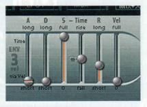
Step 5. The volume envelope has the A and D sliders (attack and decay) at zero, S (sustain) full up, and R (release) at 160ms.
