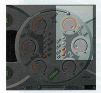
Step 4. Filter settings are simple. Move the Blend slider all the way to the right so only Filter 2 is used. Click the 24dB (per octave, the filter mode) and Fat buttons. Cutoff is all the way open, and Resonance is up just a bit to add some high frequency fizz.
