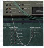
Step 3. Flip to the rear panel using the Tab key. Patch the LFO output from Mod Source into the Rotary 1 input on the back of the Combinator. This makes the LFO signal available to anything in the Combinator.
